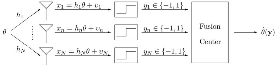
Figure 1: Block diagram for estimating a noisy measurement  $\theta$  at the fusion center when the measurement  $\theta$  is transmitted using analog communication over parallel fading channels with gains  $h_1, \dots, h_N$ . These transmissions are received by spatially separated receivers which make hard decisions that are sent to the fusion center (error free) to develop an estimate  $\hat{\theta}(\mathbf{y})$ .
